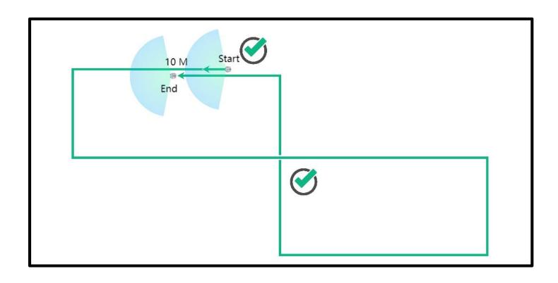
During scanning, deliberately revisit previously scanned areas to form '8'-shaped loops. Each completed loop reduces accumulated error.
