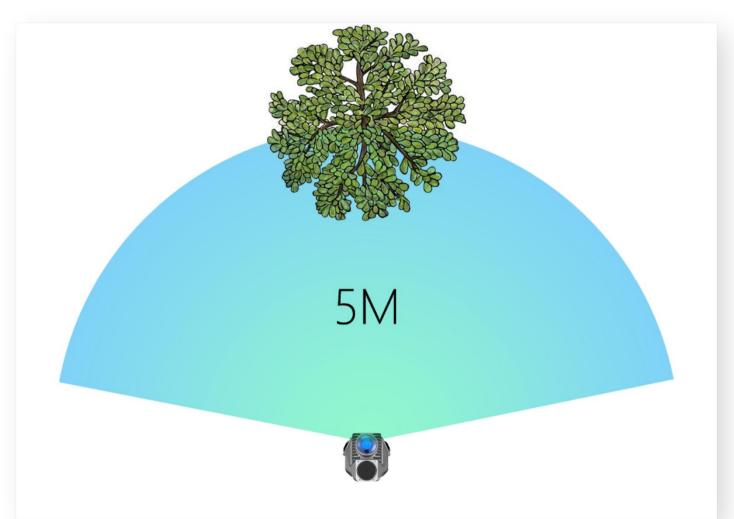
Maximum operational distance: Under optimal conditions, the S20 can capture point cloud data within a 40m range. However, in most scenarios, the LiDAR maintains best ranging accuracy within 5m-20m.
