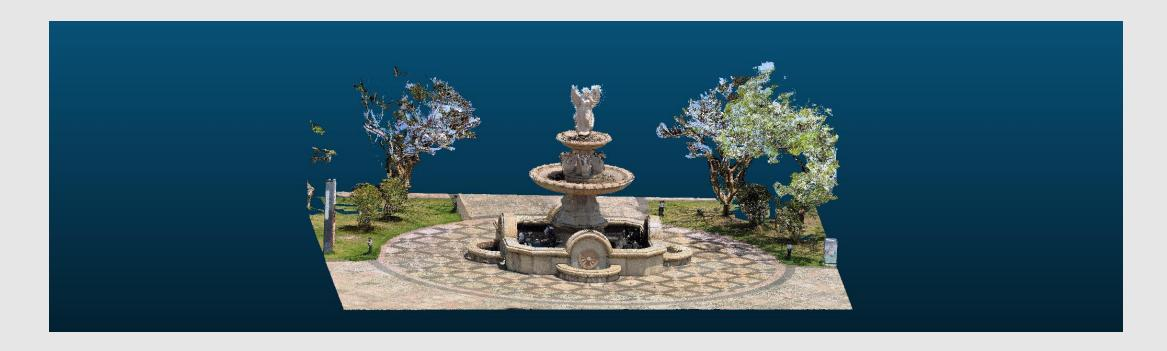
Circle around the area or object of interest. With the object or area of interest at the center, capturing from multiple angles ensures more accurate edges and more complete coloring. Alternatively, in areas with complex obstructions, images from more angles can effectively improve the completeness of the coloring.
