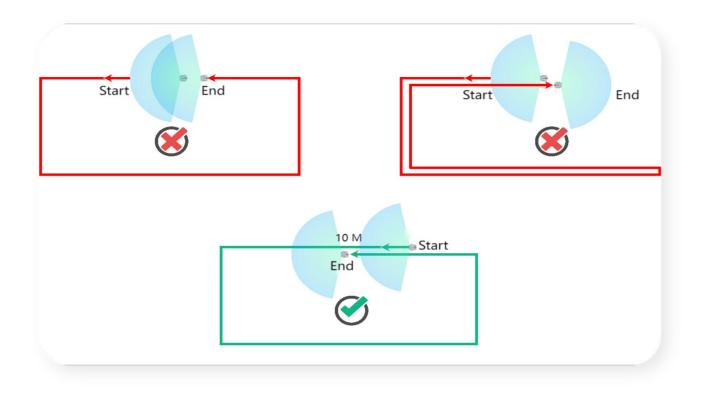
In SLAM (Simultaneous Localization and Mapping) workflows, point cloud data gradually accumulates errors over scanning time. To mitigate these cumulative errors, it is critical to implement frequent loop closures.
